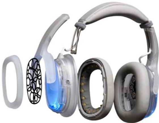
*"We needed a way to quickly churn out more parts for prototyping. Our Ultimaker machines easily handled printing half a dozen in different colors, which allowed everyone on the team to test the headphones for design, function, and usability."*
